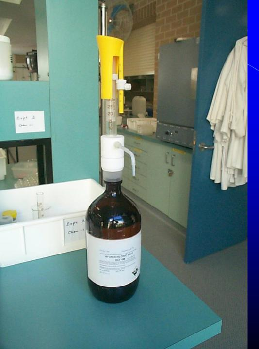
Dispensers are used in the lab and the volume you require will have been set up on the dial for you.
